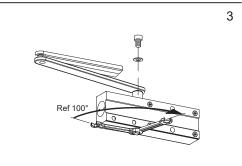
Rotate the bottom pinion to approximately 100° with a wrench as illustrated and then assemble the main arm.
