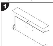
Using the templates provided, mark and drill pilot holes into the door and frame.
